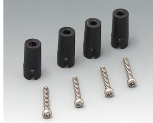
EZ031209 Extender kit ASA+PC (UL 94 V-0) black RAL 9005
