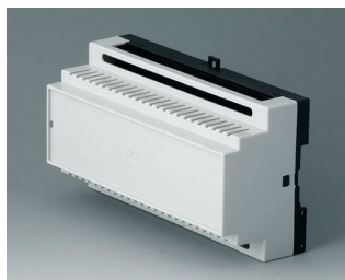
B6505114 RAILTEC B, 9 modules, Vers. I PC (UL 94 V-0) light grey RAL 7035 157x86x59mm
