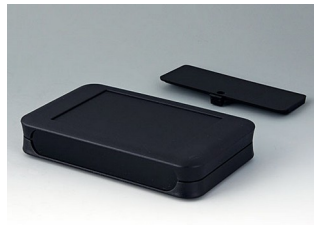
A9053219 SOFT-CASE XL PMMA (IR) (UL 94 HB) black RAL 9005 92x150x28mm IP 40
