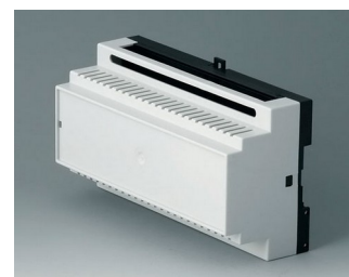
B6505118 RAILTEC B, 9 modules, Vers. IV PC (UL 94 V-0) light grey RAL 7035 157x86x59mm
