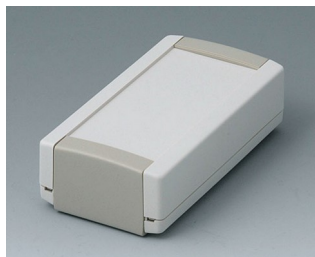
B1040365 TOPTEC 102, Vers. I ABS (UL 94 HB) off-white RAL 9002 102x54x30mm IP 40
