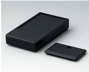
A9071209 DATEC-POCKET-BOX M PMMA (IR) (UL 94 HB) black RAL 9005 105x58x18.5mm IP 41
